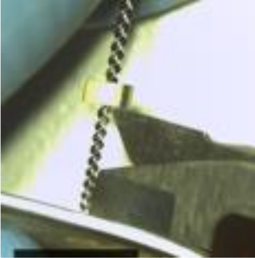
Figure 7. View under microscope of digital caliper being placed against a flat surface to measure the distance from the tip of the endodontic hand file to the stopper.
